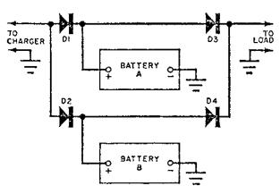
Diodes D1, D2, D3, and D4 prevent circulating current loops from being set up between batteries A and B when the batteries are connected in parallel.
