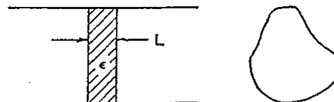
Fig. 1—Transverse dielectric slab window.
